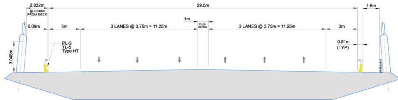
The bridge cross section was developed dependent on the roadway cross section and cable clearance. Actual cable-to-cable dimensions may vary for the cable-stayed options due to individual inclined cable geometry. The Future Design Allowance Cross Section, which represents the controlling condition, is used for the conceptual engineering phase of the project.
