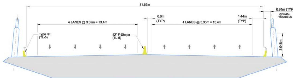
**Figure 5: Future Design Allowance Cross Section**
