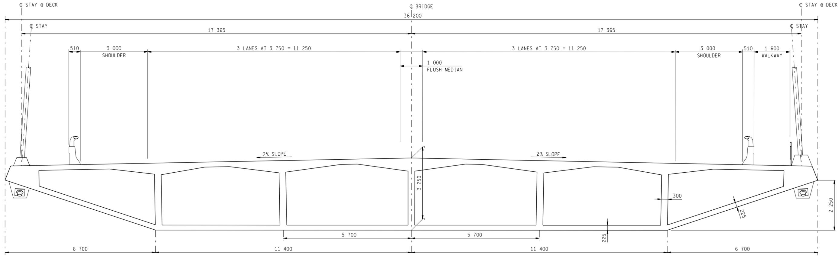
TYPICAL CROSS SECTION (CONCRETE)
